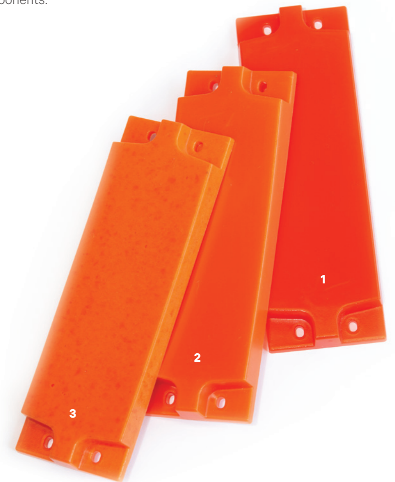
Samples of 1 virgin polyurethane 2 chemically-recycled polyurethane 3 mechanically-grinded polyurethane
